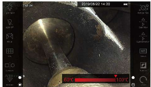
3 stage temperature warning & auto shut down function
