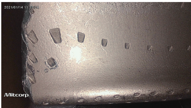
2560*1440 output by 6.0 mm HD probe (10 mm distance)
